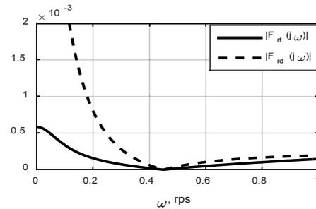
Fig. 1. Frequency responses of the transfer functions  $F_{rd}$  and  $F_{rf}$
